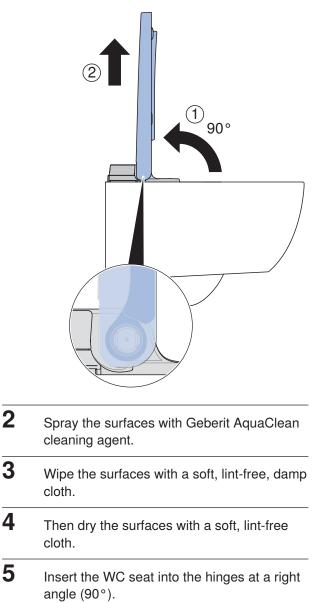
The WC seat must be positioned vertically relative to the ceramic appliance.
