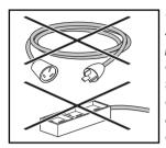
Use the specified power supply AC 220V-240V/50Hz only. Never put too much pressure on the electrical outlet. This may cause a fire or overheating. If the power cord does not suffice, please buy a professional power extension cord.
