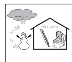
The room temperature where the product is placed should be above the freezing point. Make sure you set up the right room temperature, otherwise the product might freeze.
