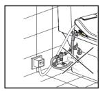
Use the attached new hose assembly during the installation. The old hose should not be reused. Do not bend or distort the inlet hose. This might cause water leakage or performance failure.
