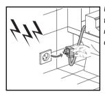
Unplug the power plug when thunder occurs. Wrong use can result in product failure or damage of the product.
