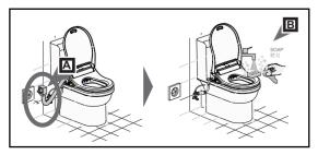
Pull the power plug out of the electric al outlet before cleaning the unit. Do not splash water directly onto the bidet. Failing to do so might cause an electrical shock.
