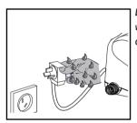
Do not touch the power plug with wet hands. This might cause a fire or an electrical shock.
