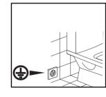
Check if the type C electrical plug is connected to the ground line. Make sure the electrical plug is plugged into an outlet that is properly installed and grounded. Electrical power supply should be implemented by a qualified electrician or service technician. Improper use of the grounding plug can result in electric shock.
