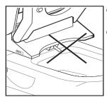
Do not bend or distort the nozzle. This might cause product damage or performance failure.
