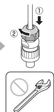
**3** Installing the bowl unit (see bowl unit installation guide)
