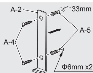
When mounting on a plaster board or tiled wall.
